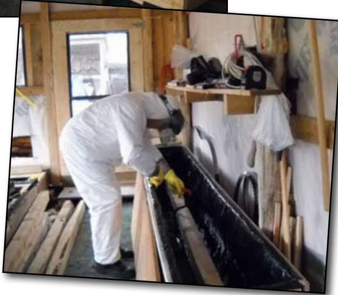
Photo 5 (right) - Always wear protective clothing to prevent chemicals from getting on you or your clothing. And always keep your tanks covered, whether in use or not, to keep rain, debris and animals out.
